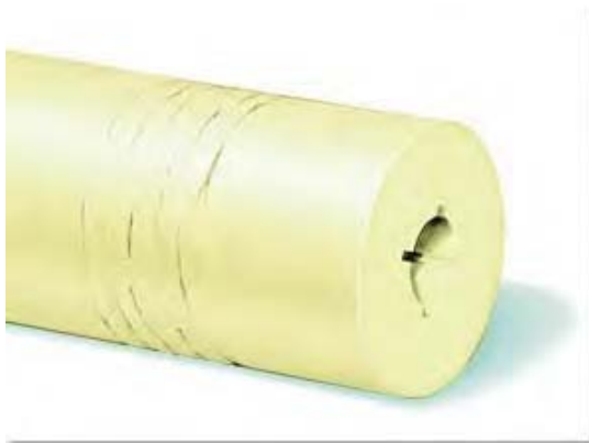
(1) Cracks in the roller surface indicate a damage in the entire structure.
