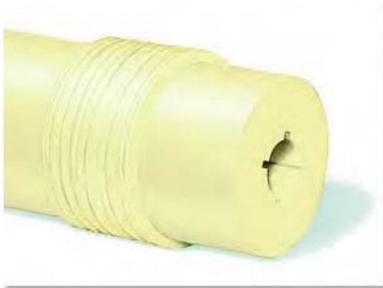
(3) The removed areas are replaced by new mill roll inserts.
