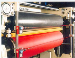
Küstner calender - Heat and pressure resistant MITEX KALANTEC covering 75 Shore D
