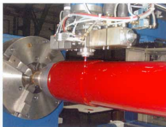
Ribbon flow casting machine - Production of high performance elastomer coverings
