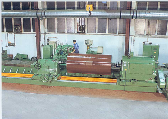
Heavy duty grinding machine for precision roll grinding
