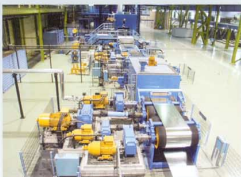
ThyssenKrupp Nirosta S-Rolls - Annealing and Pickling Line (APL)
