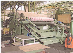
Voest coilcoating equipment with MITEX roller covering ULTRAMAX
