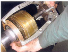
Special equipment for the removal of bearings
