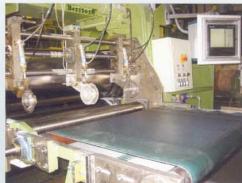
High performance calender equipped with modern measuring equipment
