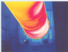
Heat distribution measurement in high performance rollers, shown with special R&D equipment
