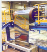
MITEX non-slip roller covering ULTRADUR in deflector roll positions in the new APL
