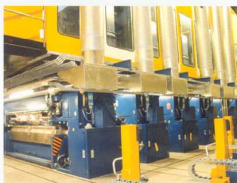
Cerutti printing unit - gravure printing width 3600 mm equipped with MITEX impression roller coverings
