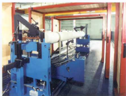
Schenk dynamic balancing machine for roller coverings
