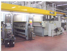
Schiavi - Packaging gravure press IDEA 1880 mm printing width
