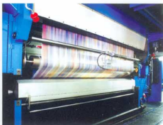
MITEX impression roller covering in 3650 mm KBA gravure printing unit at 15 m/s
