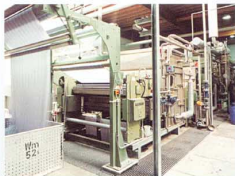
Küstlers - Wet treatment with MITEX textile roller coverings
